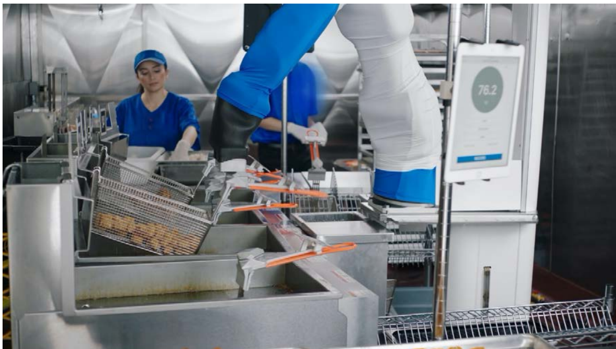
'Flippy', an autonomous robotic kitchen assistant that can learn from its surroundings and acquire new skills over time. Shown at work in a kitchen alongside 'co-workers' helping to fulfil customers' orders (Courtesy to "Miso Robotics").
